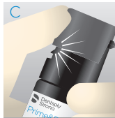
To close the Bottle, press down the cap until it locks in place with a perceptible click.
