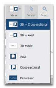
Using the View dropdown from the toolbar, you can choose to combine the 3D view with the cross-sectional or the axial images; or you can also visualize the cross-sectional, axial images or panoramic images in full screen.
